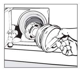
Unscrew the fluff filter completely and then clean it thoroughly.
